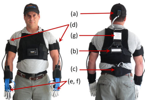
Fig. 1 Front and back views of the wireless Measurand ShapeWrap III upper-body motion capture system, showing (a) a head orientation sensor, (b) a thoracic orientation sensor, (c) a pelvic orientation sensor, (d) two arm sensors, (e) four finger sensors for each hand, (f) a thumb sensor for each hand, and (g) the data concentrator
